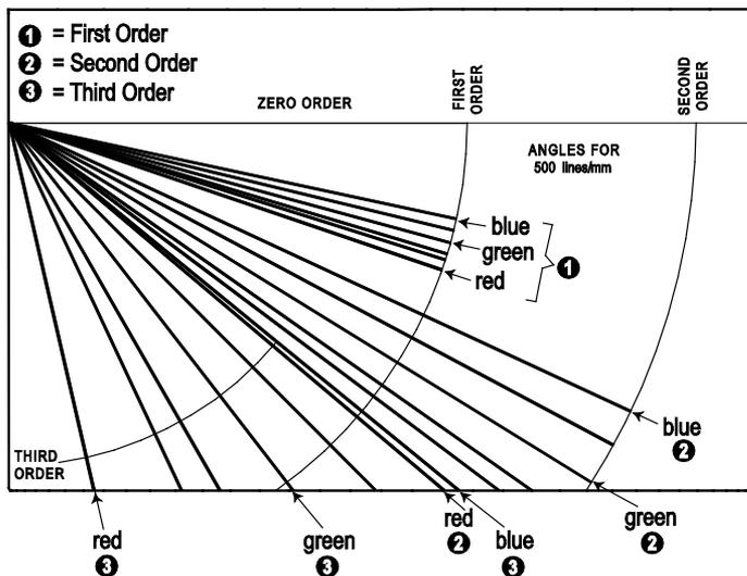
Zero order (looking straight at the light) follows a path that does not change angle when passing through the grating. You can view the first, second and possibly the third, order angles for each spectrum by looking along the lines on the cardboard
