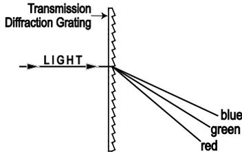
Zero order (looking straight at the light) follows a path that does not change angle when passing through the grating. You can view the first, second and possibly the third, order angles for each spectrum by looking along the lines on the base plate. Negative first, second and third order are on the other side of zero order (a mirror image of the positive orders).
